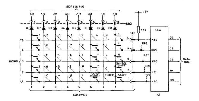
When the keyboard scanning routines are entered the CPU performs successive I/O read cycles setting the IOREQ and RD lines to the ULA, low. At the same time, the I/O port addresses placed on the upper half of the address bus are modified with each cycle such that each of the address lines A15 through A8 is set low in turn, the other lines remain high.
