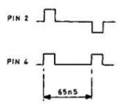
If IC14 pins 2 and 4 are correct, change modulator.
